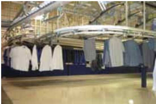
Figure 2: Autosort Garment Sortation Machine. Barcode labels allow garments to be automatically sorted by Cintas Route Truck, Delivery Date, Customer and Employee.
