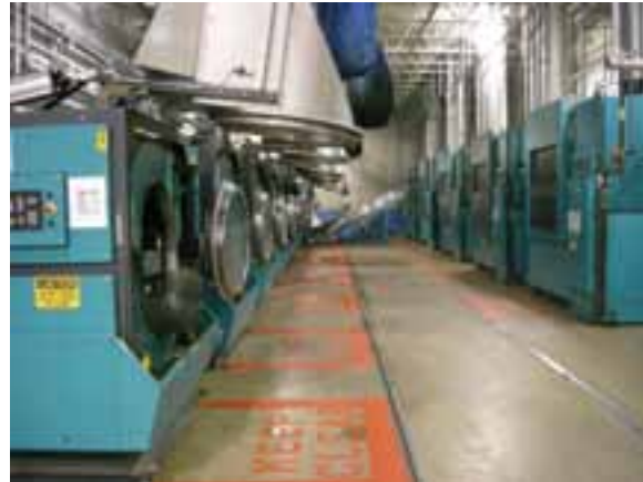
Figure 1: One of 150 Cintas Wash Alleys located throughout the U.S. and Canada. Tilttable Washers (left), Dryers (right), Movable Shuttle Conveyor (background) and Chute (overhead).
